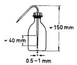
Fig. 1. Polyethylene weighing burette for NaOH solution. Over a length of 4 cm, the end of the spraying nozzle inside the bottle is extruded to an inside diameter of 0.5-1 mm.
